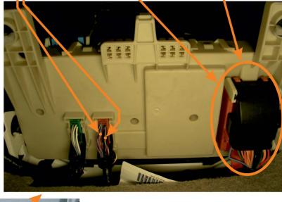
CEM MODULE (under glove compartment - passenger's side)
