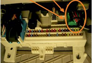
green/blue pin9 green connector 41PIN (blockade circuit)
