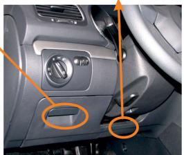
(blinkers sequence steering - emergency light switch) brown connector "C" 52PIN purple pin7
