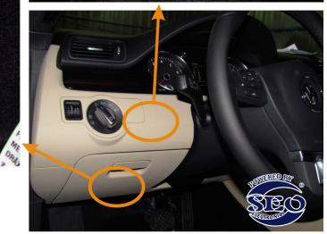
(alternative control blinkers - emergency light switch) brown connector "C" 52PIN brown pin7
