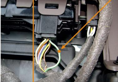
(blinkers sequence steering - emergency light switch) black connector 12PIN green-white pin10
