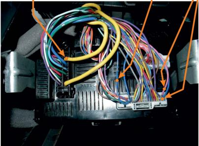
(blinkers sequence steering - emergency light switch) white connector 40PIN blue pin26
