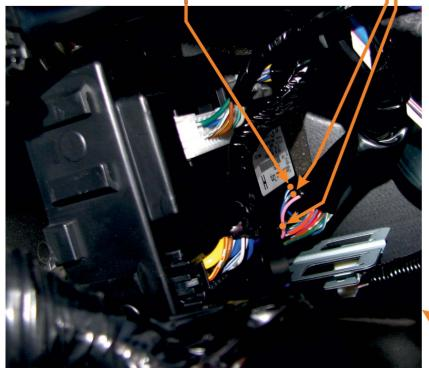
(blinkers sequence steering - emergency light switch) black connector M68 40PIN blue/white pin29
