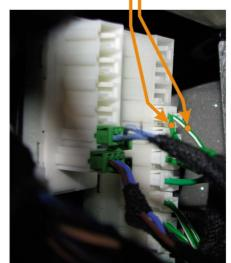
LEFT BLINKER white connector 48PIN on SAM module (left side of steering column)
