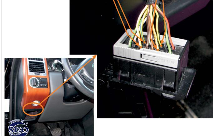
(blinkers sequence steering - emergency light switch)
