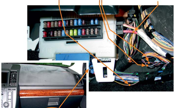
(blinkers sequence steering - emergency light switch) blue connector 76PIN brown/yellow pin8
