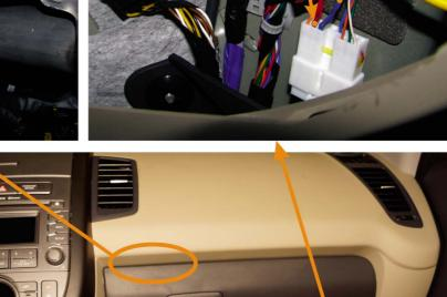
(Alternative control blinkers - emergency light switch) white connector 24PIN blue/black pin12
