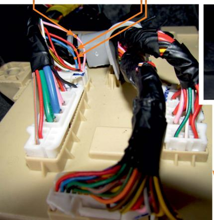
red-white pin5 black connector 8PIN (blinkers sequence steering - emergency light switch)
