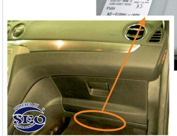
MODULE (under glove compartment - passenger's side)
