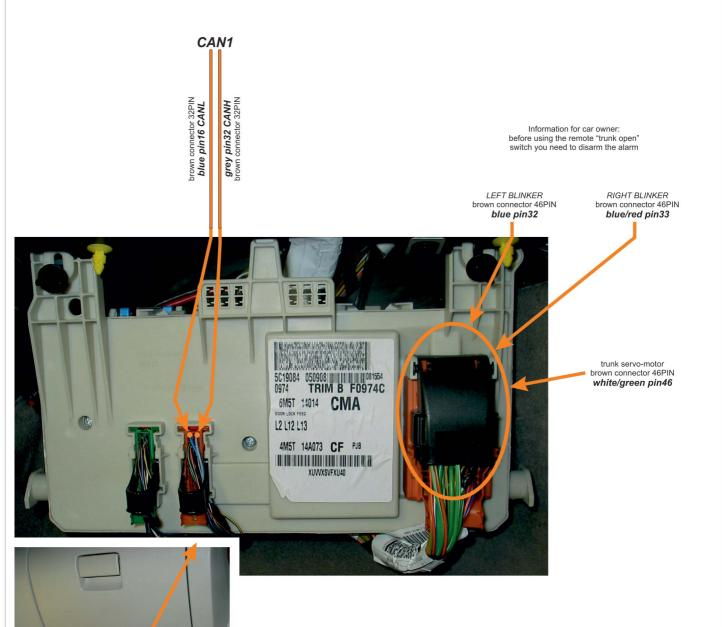
MODULE (under glove compartment - passenger's side)
