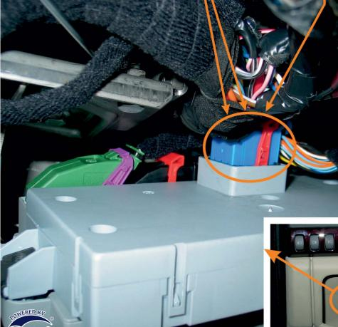
STARTER'S BLOCKADE CIRCUIT red/black pin8 black connector 24PIN - module on bottom of steering column
