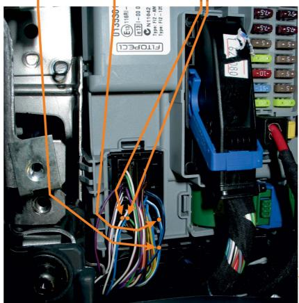
RIGHT BLINKER black/blue connector 60PIN (module front) blue/white pin10
