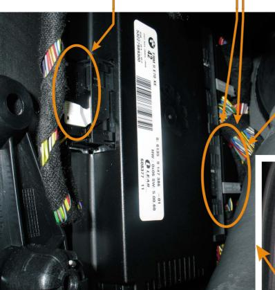
(alternative control blinkers - emergency light switch) black connector 26PIN brown/blue pin18
