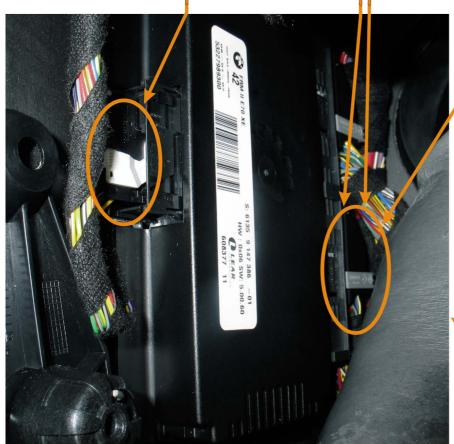
(alternative control blinkers - emergency light switch) black connector 26PIN brown/blue pin18
