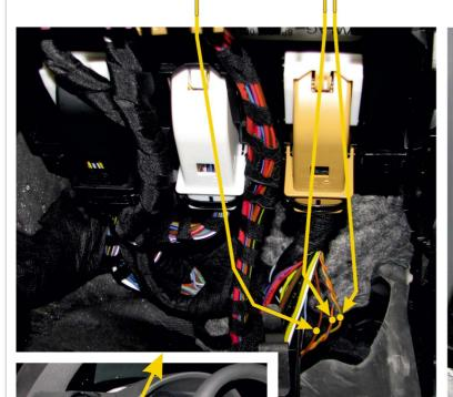
(alternative control blinkers - emergency light switch) brown connector "C" 52PIN brown-red pin7
